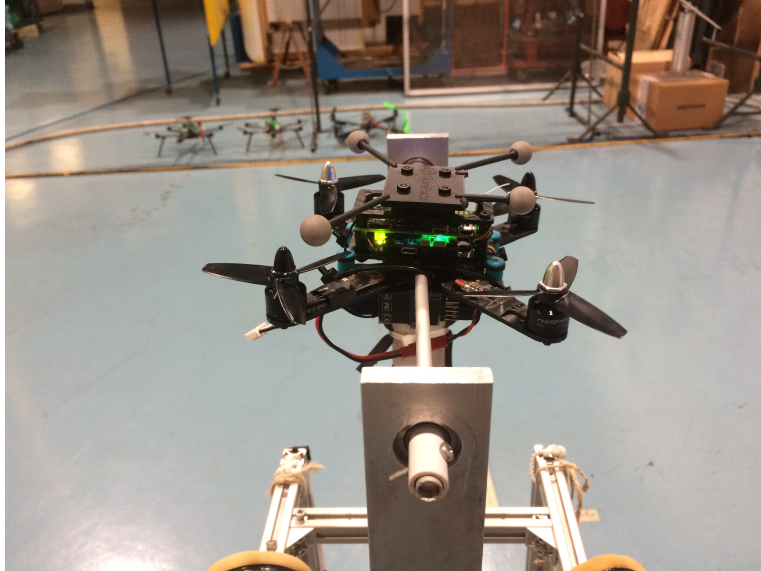
Figure 5.5: The ANT-1 quadrotor on the test-bed.
