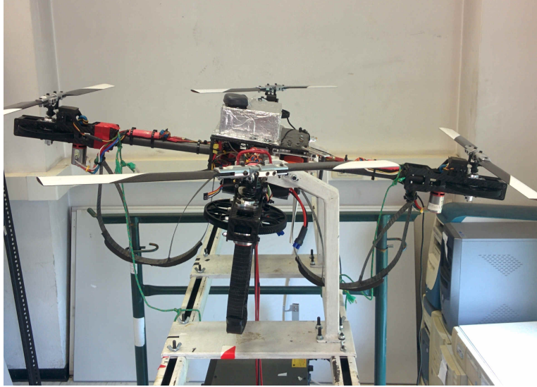
Figure 5.1: Aermatica P2-A1 on laboratory test-bed.
