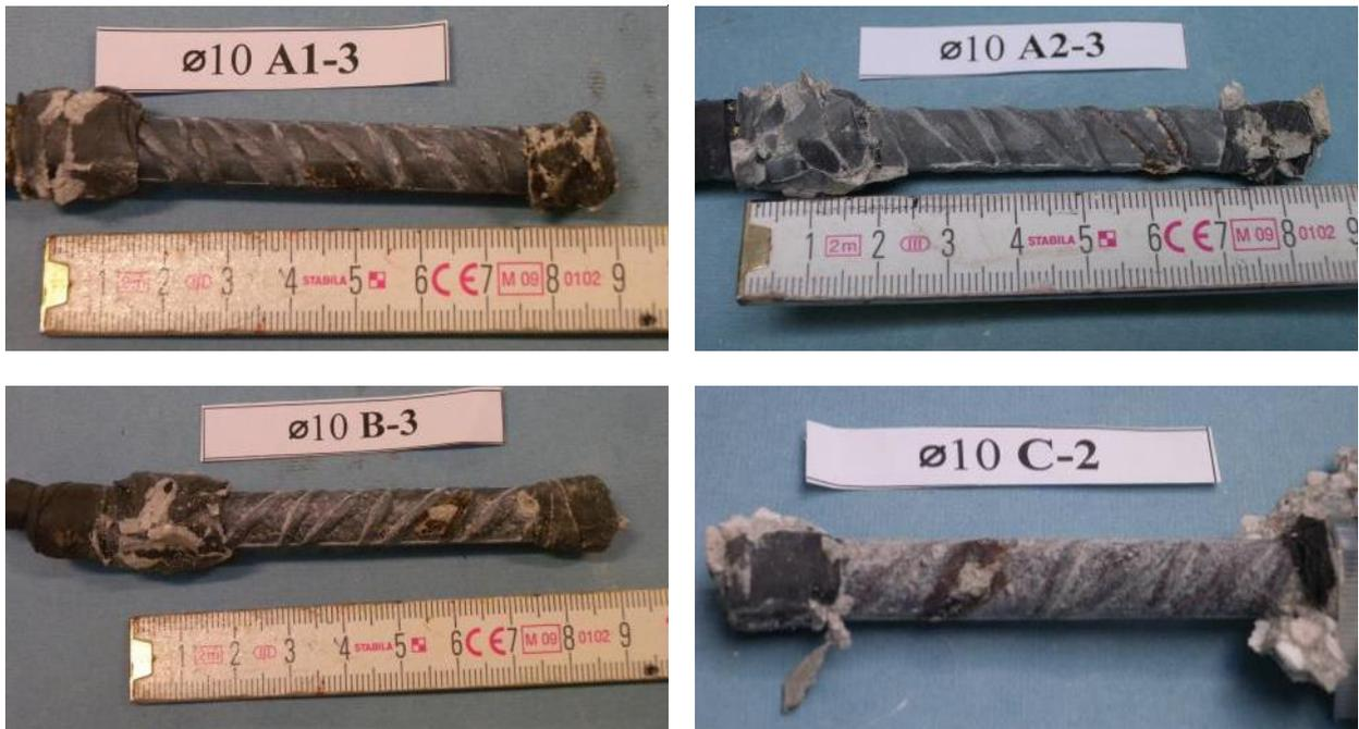
**Figure 4.23** The surface condition of 10 mm diameter steel bars with different initial surface conditions removed from the splitted reinforced specimen. (A1:as-received; A2:sandblasted; B:exposed for 6 months; C:exposed for 1 year)
