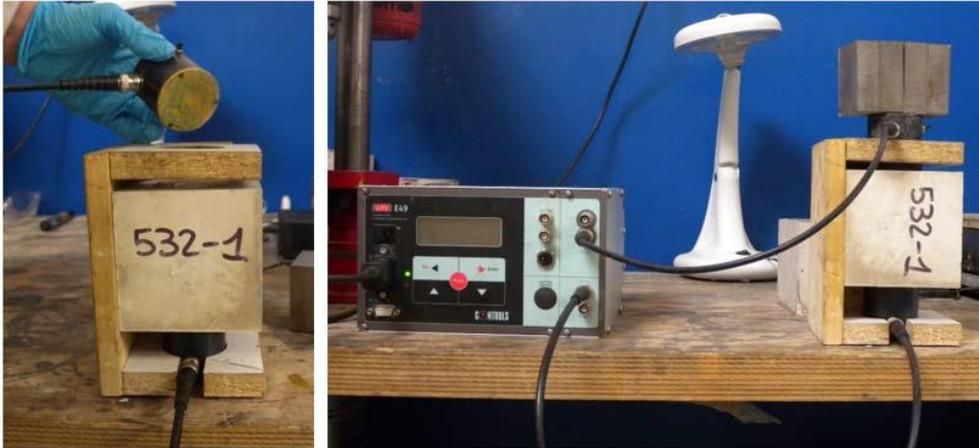
**Figure 2.5** Ultrasonic test setup for cubic concrete sample.
