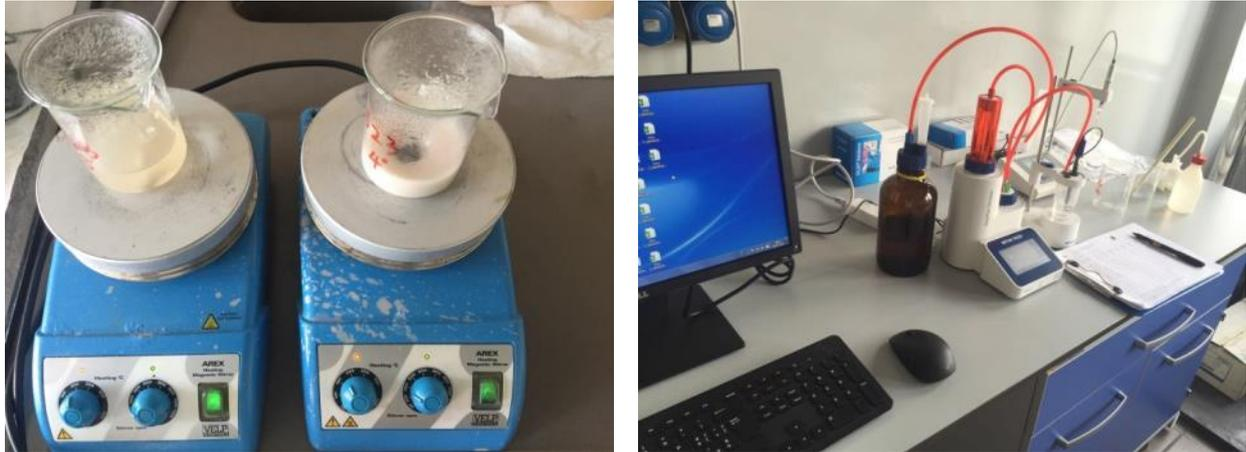
**Figure 2.10** Chloride content analysis for CSA-based concrete.
