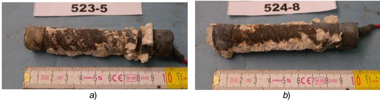
**Figure 4.27** The surface condition of carbon steel in 0.55 w/c ratio carbonated CSA-based concrete a) without chloride and b) with 0.4% chloride made with SL05 NF cement.
