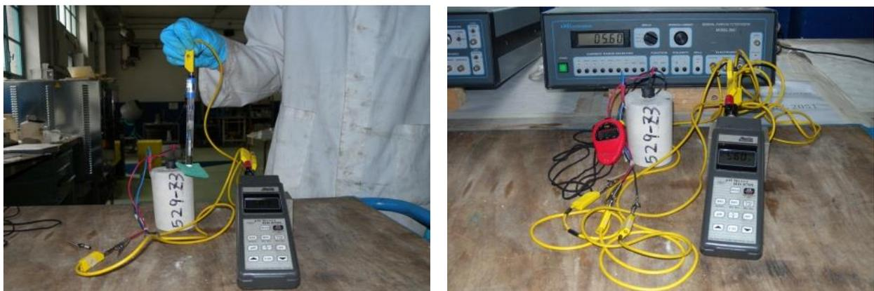
**Figure 2.13** Corrosion potential and corrosion rate measurements.
