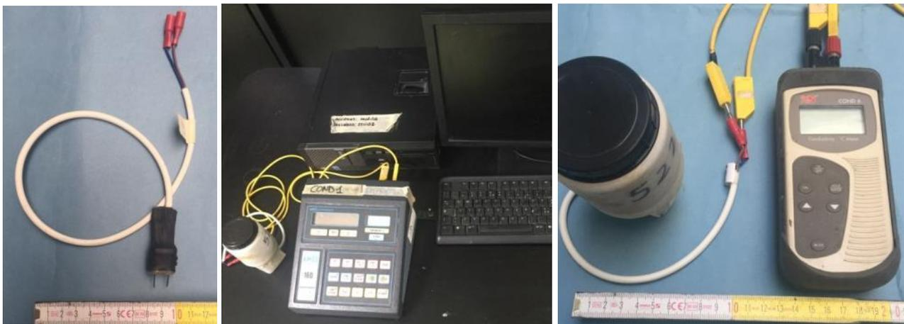
**Figure 2.7** A handmade resistivity probe and conductance tests.
