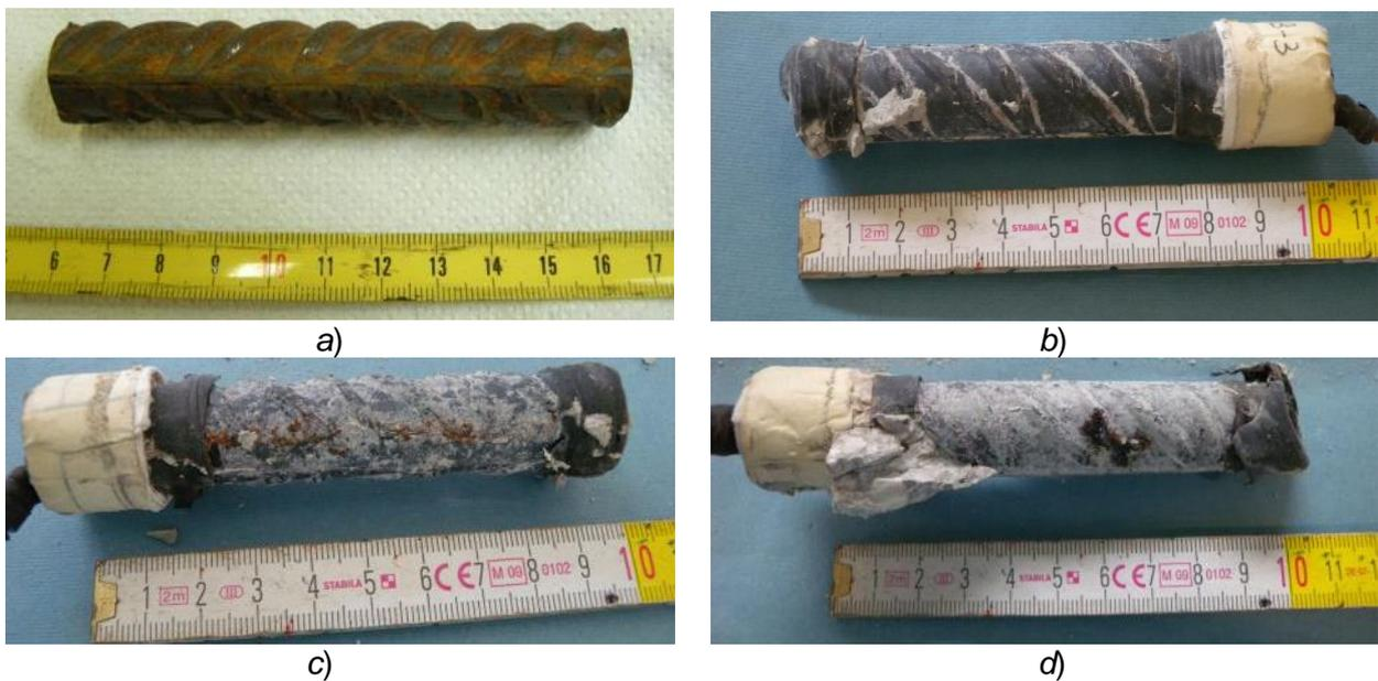
**Figure 4.24** Surface condition of steel bars with 18 mm diameter labelled “B-3” a) before casting and b) after splitting (pitting spot on the other side), c) “C1-3” and d) “C2-3”. (B:exposed for 6 months; C1 and C2:exposed for 1 year)
