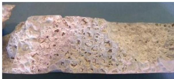
**Figure 4.9** Cracked surface of expanded glass mortar (specimen M137) subjected to ASR test. M137:100% standard sand replaced by expanded glass.
