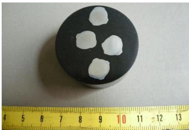
**Figure 2.4** A sample for metallographic analysis of pre-oxidised and sandblasted steel bars.
