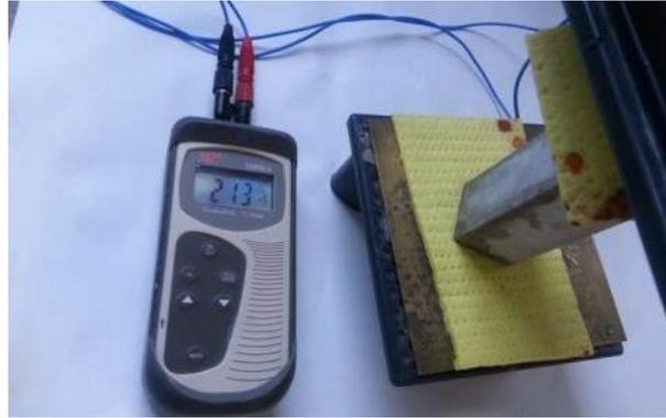
**Figure 2.6** Conductance test on prism sample.
