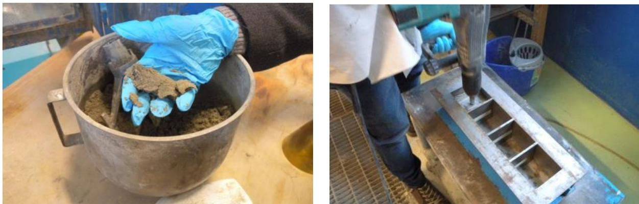
**Figure 2.3** Preparation of cement-stabilised rammed earth specimens.
