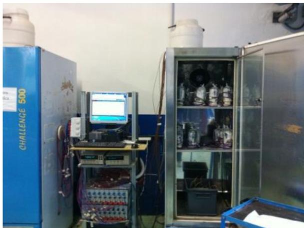
**Figure 2.12** Climatic chamber and data logger setup used for corrosion tests.
