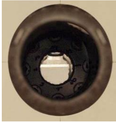
Figure 4.5: Vapor bubble and liquid phase inside equilibrium cell.
