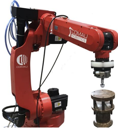
Figure 2.6: Implicit force control experimental setup.
