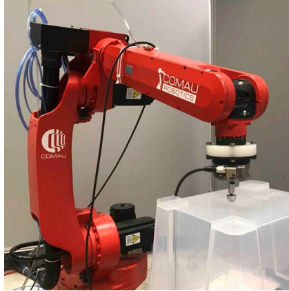
Figure 3.9: Experimental setup: plastic environment ( K_E \approx 10^4 \text{ N/m} )
