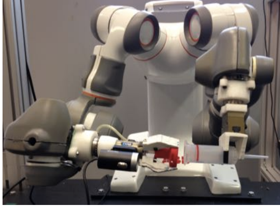
Figure 6.15: Experimental setup: the ABB YuMi robot used in this thesis has been equipped with Schunk pneumatically actuated grippers and 3D printed tools, specifically designed to perform a cap rotation task using an Eppendorf combitip ® plastic pipette.
