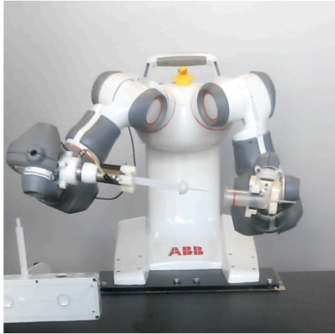
Figure 6.8: Experimental setup: the ABB YuMi robot used in this thesis equipped with Schunk pneumatically actuated grippers and 3D printed tools to perform the peg-in-hole insertion of an Eppendorf combitip® plastic pipette.
