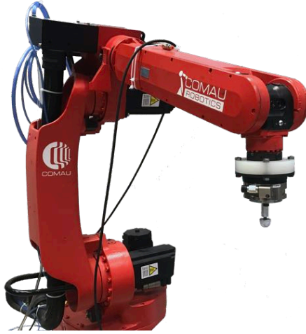
Figure 2.4: The COMAU Smart Six, 6 kg payload position controlled industrial manipulator, used for experimental validation.
