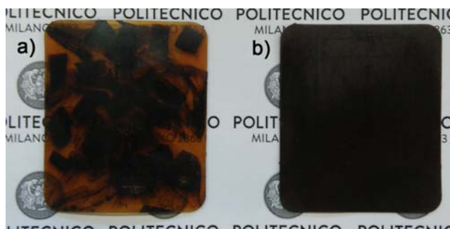
Figure 18. Photographic image of molds of (a) PU/IND and (b) PU/NL composite systems at 10 wt.% filler loading.
