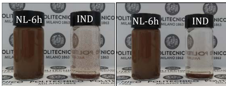
Figure 4. Photographic images of water dispersions of ultrasonically treated NL-6h and pristine IND lignin (a) after dispersion process and (b) after 15 months at rest.
