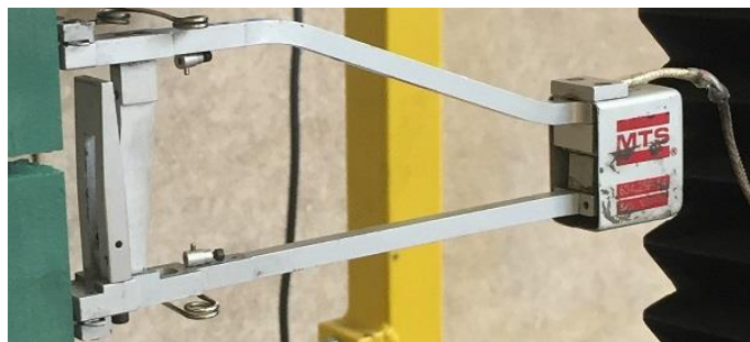
Figure 2. 11: extensometer used for measuring the displacement of the specimen during the tensile tests.
