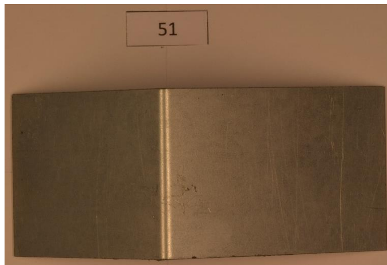
Figure 4. 22: specimen 51 bent with die Necuron 1150 with no defects.
