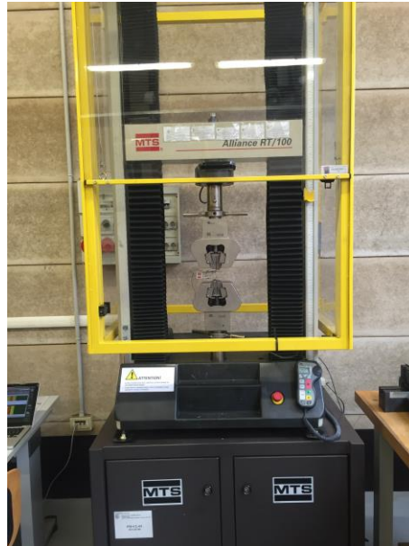
Figure 2. 10: tensile tests machine MTS Alliance RT/100.
