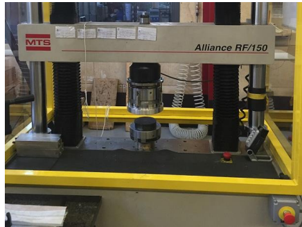
Figure 2. 13: machine used for the compression tests.
