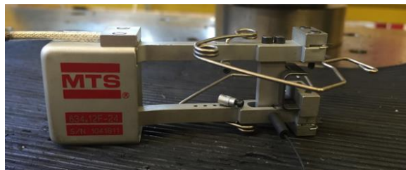
Figure 2. 14: extensometer used for compression tests.
