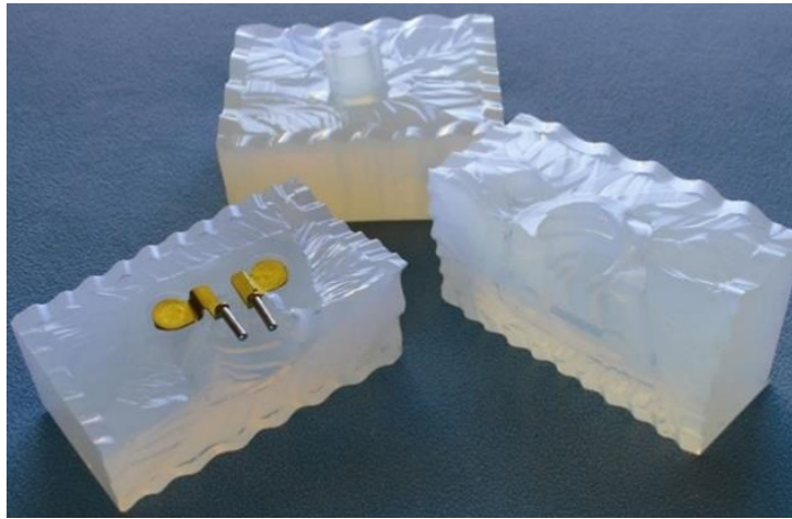
Figure 1. 18: industrial example of epoxy moulds [31].
