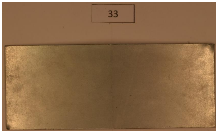
Figure 4. 20: specimen 33 bent with drilled rubber tool with no defects.
