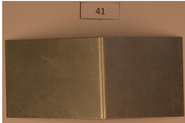
Figure 4. 21: specimen 41 bent with die Necuron 1050 with no defects.
