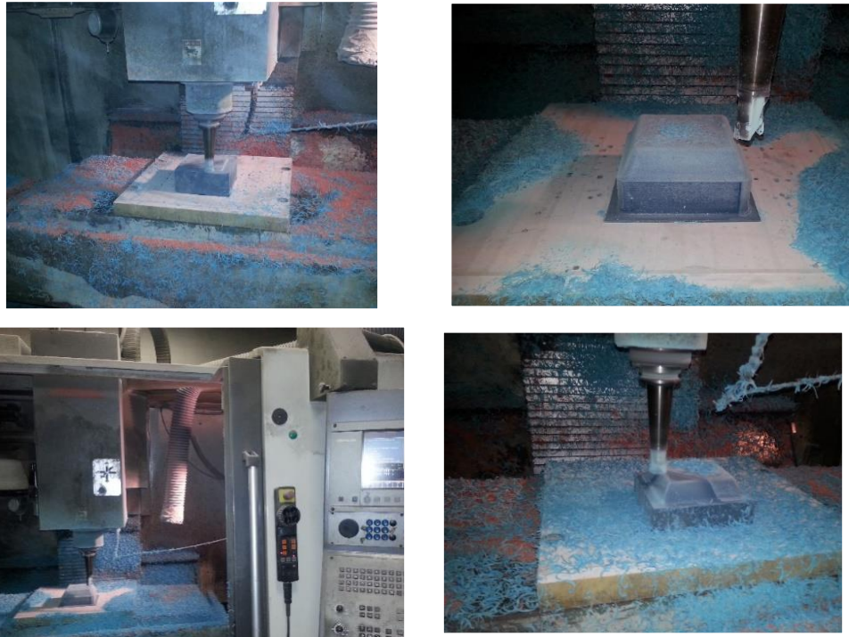
Figure 3. 56: milling operations performed for making the punch.
