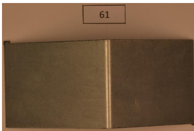
Figure 4. 23: specimen 61 bent with die Necuron 1300 with no defects.
