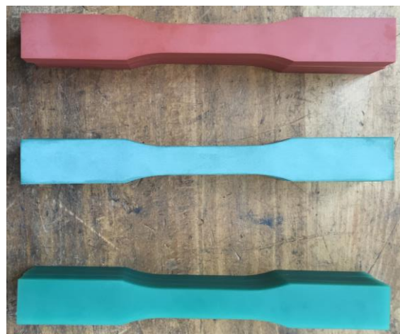
Figure 2. 9: experimental tensile specimen of Necuron 1300 (red), Necuron 1050 (light green), Necuron 1150 (dark green).
