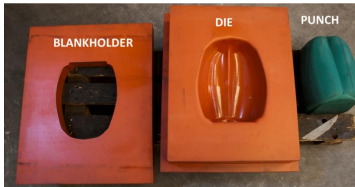
Figure 1. 23: industrial application of resin tools [43].
