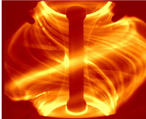
Figure 1.7: Plasma discharge in the Tokamak MAST. ELMs are identified by the plasma filaments that are visible in the image. Figure taken from [19].
