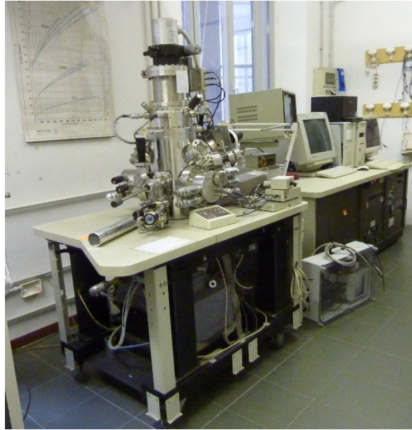
FIGURE 39 – THE SCANNING AUGER MICROSCOPE MODEL 660 BY PHYSICAL ELECTRONICS BEFORE THE UPGRADE
