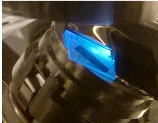
FIGURE 109 – OPTICAL PICTURE OF A MAGNESIUM OXIDE BULK SAMPLE OPTICALLY EXCITED WITH PHOTONS OF 3.6 eV
