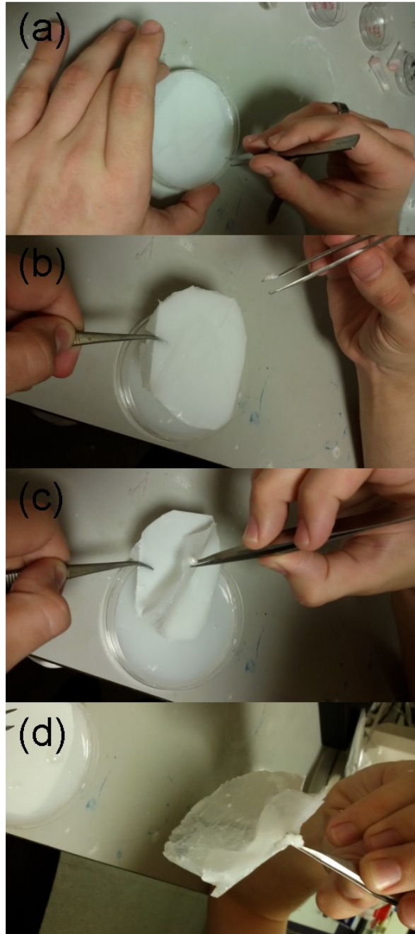
Figure 4.9: The teflon assisted method for liquid to air interface film removal, (a) physically separate the film from the outer rim of the dish, once complete (b) lift the teflon with the film and mesh on top, draining partially the excess solution. (c) use a separate tweezer at a higher angle to separate the film from the teflon continuing to drain the excess. (d) remove and set film to dry.
