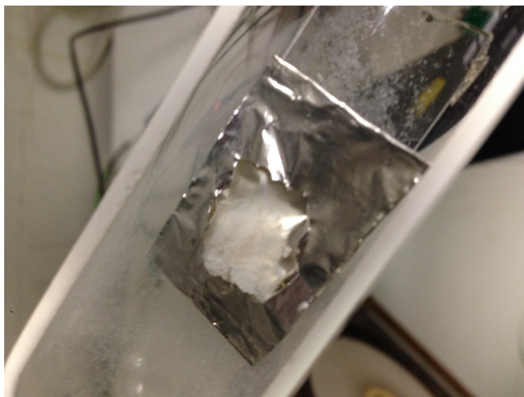
Figure 4.13: LTA calcined film within aluminium holder.
