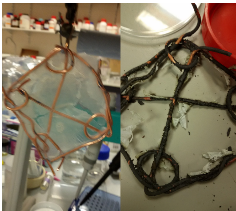
Figure 4.5: Homemade copper-based removal tool to remove larger areas and to calcine together with the film before calcination (left) and after calcination (right).
