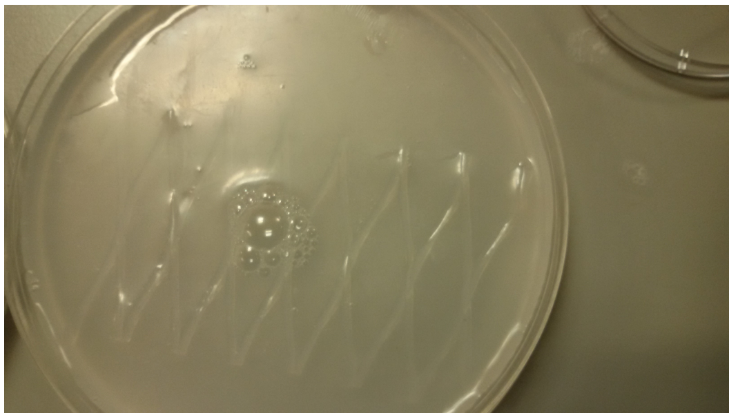
Figure 4.2: Solution freshly poured into a Petri dish with plastic mesh placed at the bottom.
