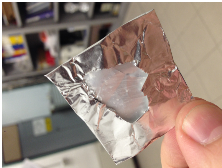
Figure 4.12: A cut piece of LTA film encased in aluminium holder, prior to calcination.
