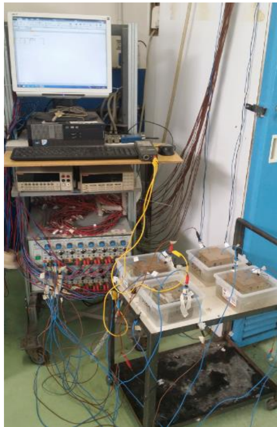
Fig. 3.7 Test set up for potential-static electro-chemical test
