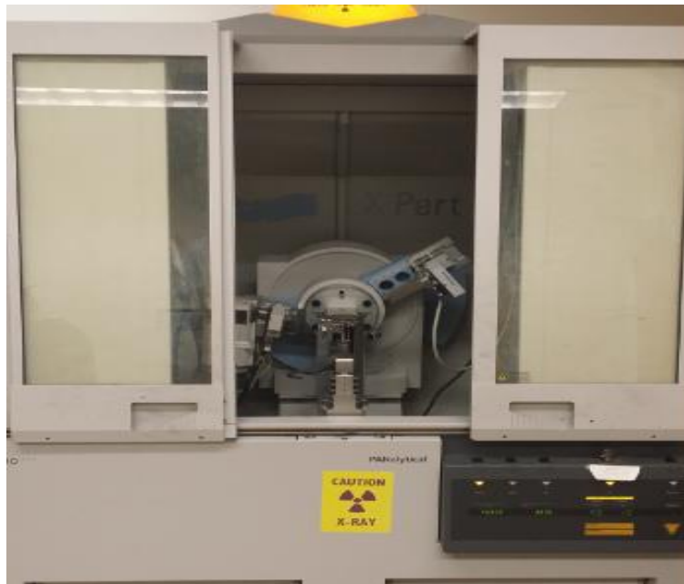
Fig. 3.12 The test setup for X-rays diffraction test
