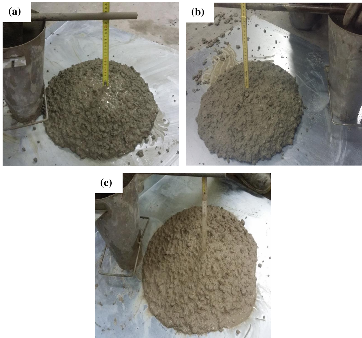
Fig. 5.1 Appearance of fresh concretes in slump test: (a) OPC mix, (b) OPC25-CSA50-SL25 mix, (c) CSA-DHE1 mix
