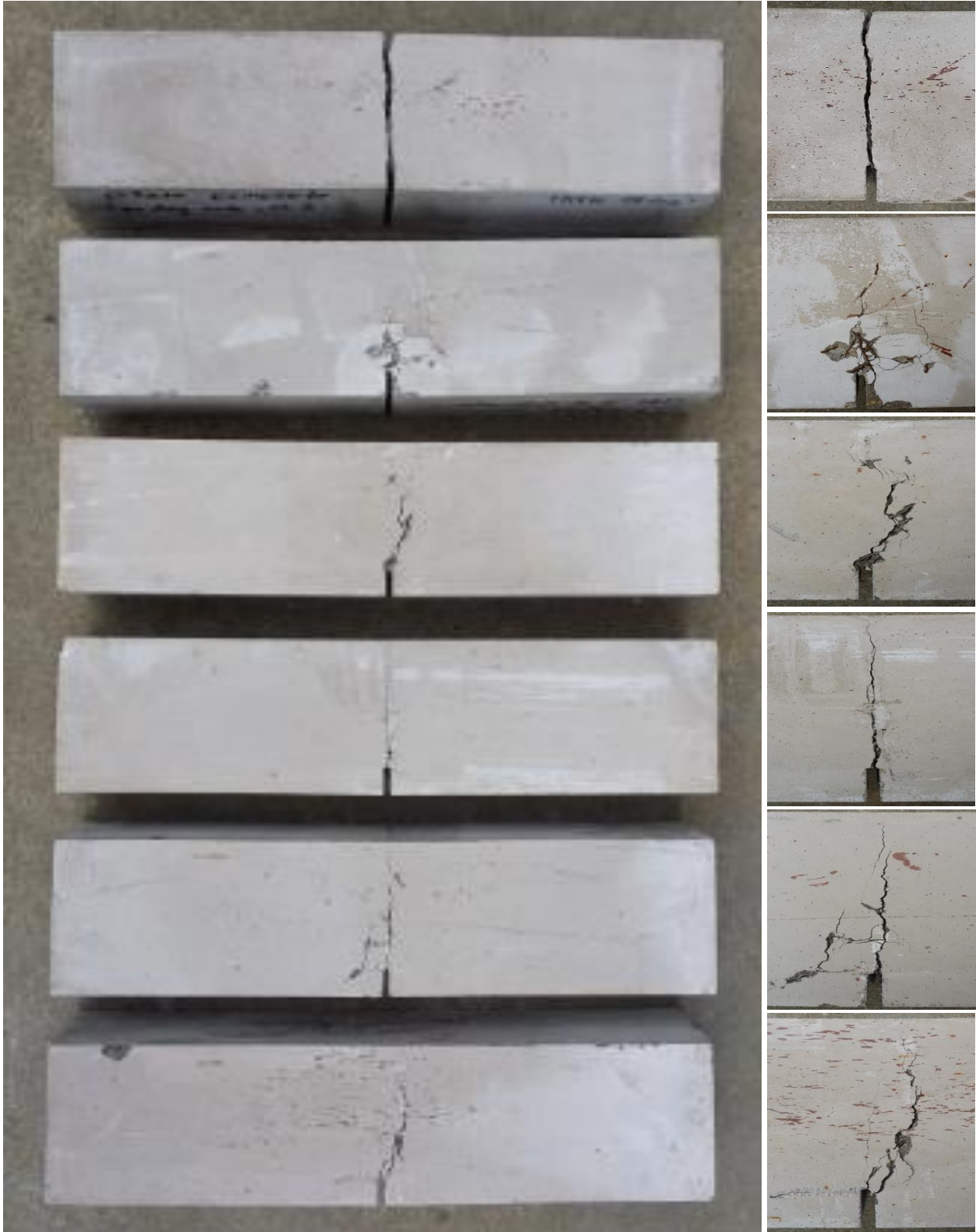
Fig. 6.33 Cracks propagation on the surface of concrete beams reinforced with different type and hybridization of fibers (close-up of cracks propagation are shown in right side of each beams)
