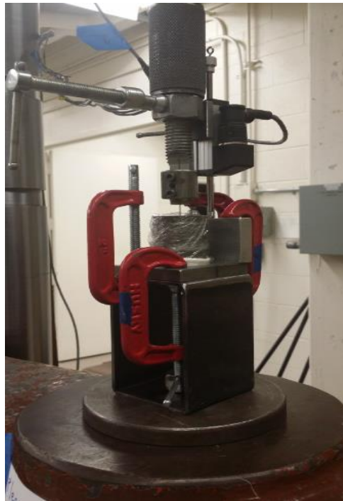
Fig. 3.8 Test setup for single fiber pullout test
