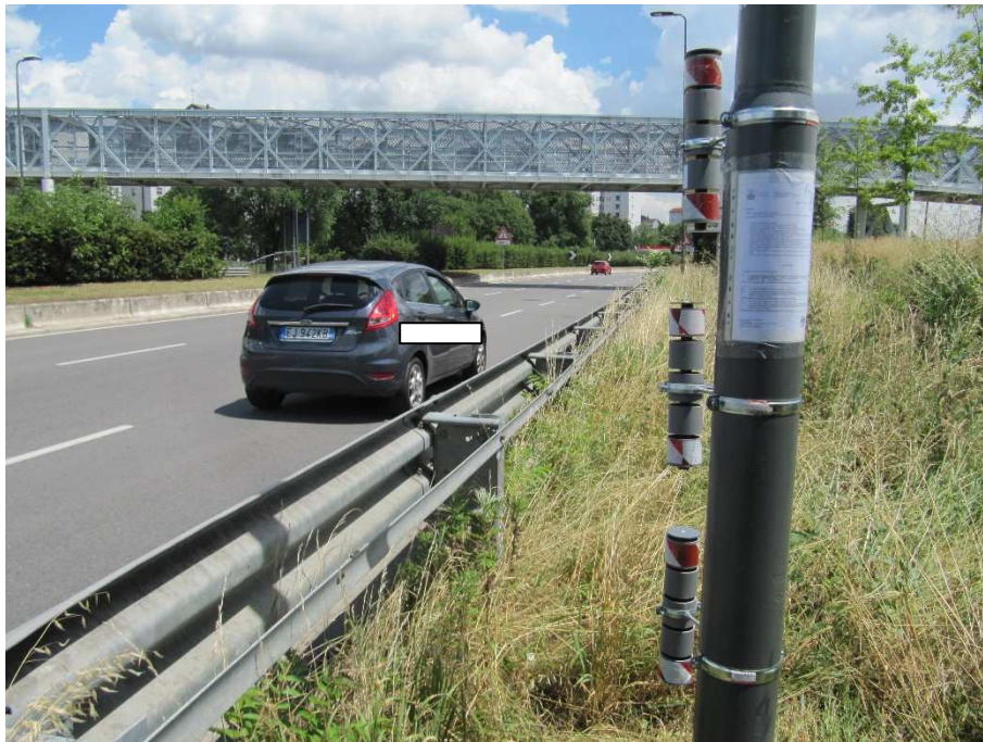
Figure 36. Example of passive sampler installed in Via Parri
