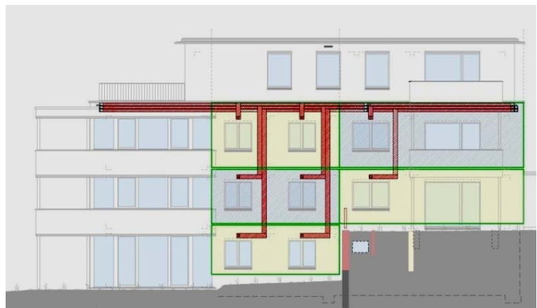
Figure 4 - Ventilation distribution on south-east façade
