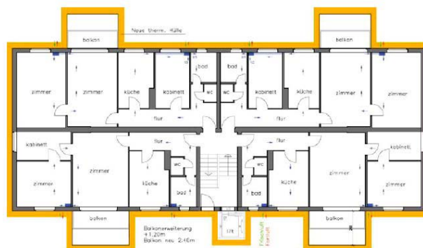
Figure 3 - Exemplary floor plan of renovated building – showing new thermal envelope, integrated balconies and new lift (Source: Hohensinn ZT GmbH)
