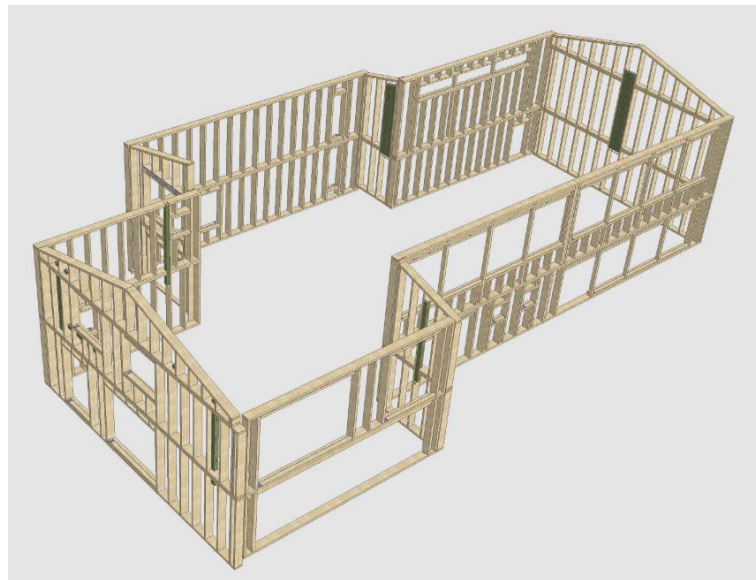
Figure 3 - 3-D sketch of the timber frames, also showing the integrated ventilation pipes (source: Renggli HolzbauWeise)
