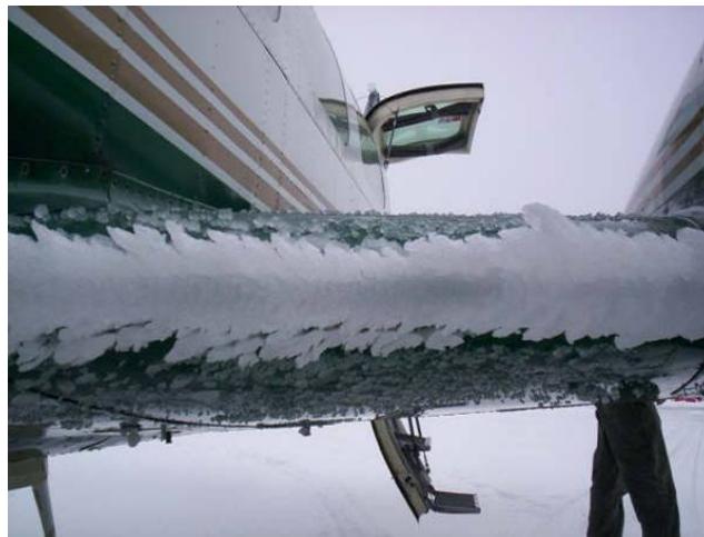
Figure 1.6: Example of rime ice accretion from Ref. [13].
