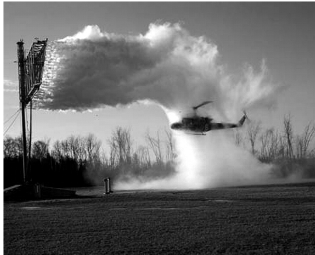
Figure 1.1: In-flight ice accretion testing on a rotorcraft. Ref. [7]
