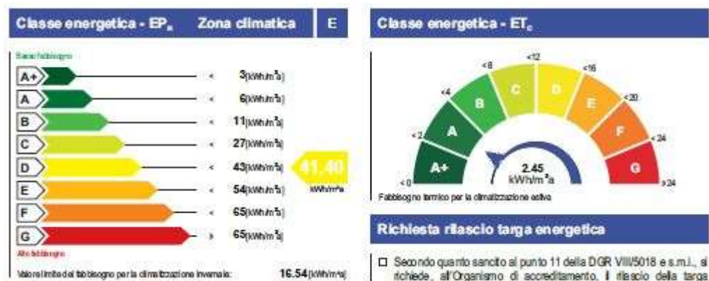
Figure 4.4.9 Energy Performance Certificate sample showing a difference between Winter and Summer Energy Labels
