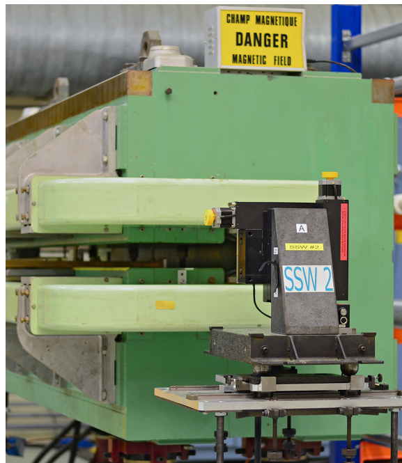
Figure 6.1: Single-stretched-wire system, in translating mode, mounted on the MCB22 reference dipole magnet.
