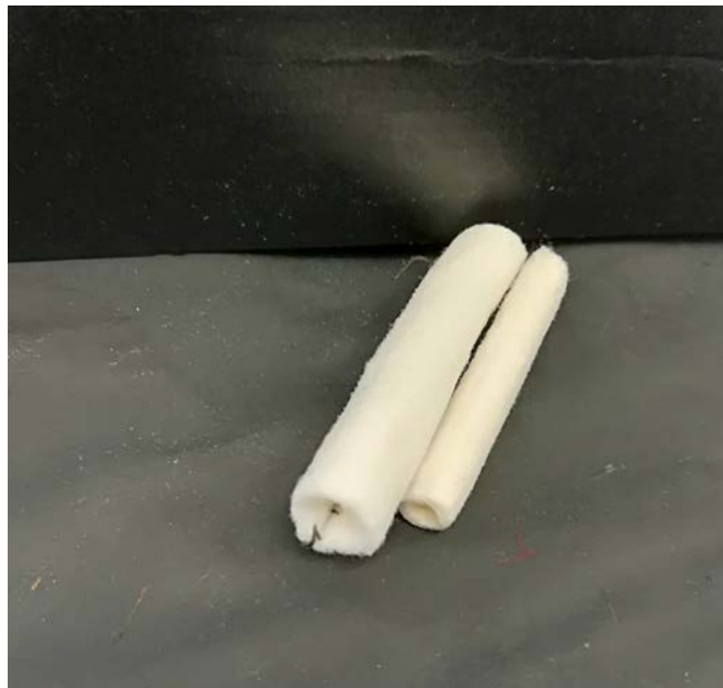
Figura 25: Scaffold in PGA/PLLA.
