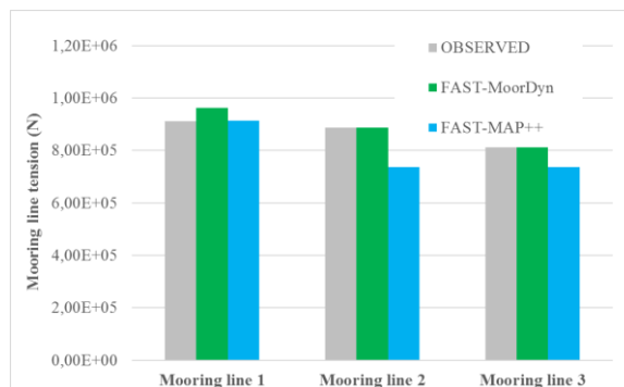
Figure 6.15. Test 1380: mean between maximum and minimum value of the three mooring lines tensions.
