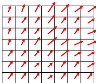
Figura 2.2: The Vector Field (VF) is a possible transformation involved in registration. VF is a grid superimposed to the point cloud, in which each block has associated a displacement vector, representing the direction and the intensity applied to what is inside that block.
