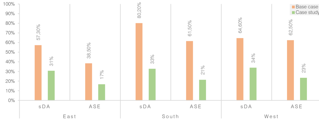
Figure 77 - Comparison between the un-shaded building with the case study based on the achieved sDA and ASE for each orientation simulated
