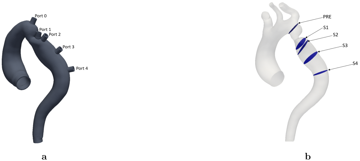
Figure 32: 3D model used in the in vitro setup with ports for pressure transducers (a) and corresponding cross-sections in the computational domain (b) (referred to as S1-S4).
