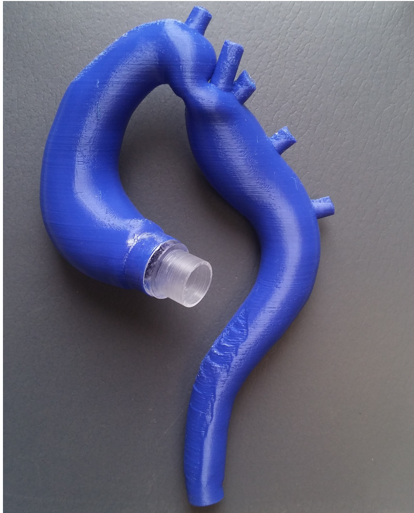
Figure 2.20: 3D printed of the aorta with connection ports.
