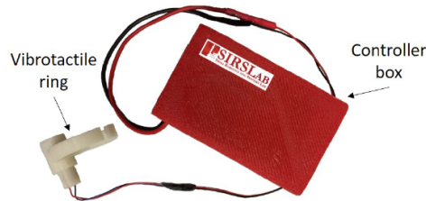
Figure 7.2: Illustration of the vibrotactile ring realized by the University of Siena. This ring can during the experiment is worn on the operator's left hand and the controller box is attached to the Velcro bracelet worn on the operator's left forearm. The communication with the ring is wireless
