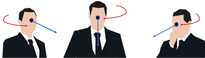
Figure 4.12: When a human decides to shift its focus from one objective to another one, the z_{HeadVector} changes direction and helps clarifying the intended goal. This change in head orientation occurs slightly before the corresponding hand reaching motion
