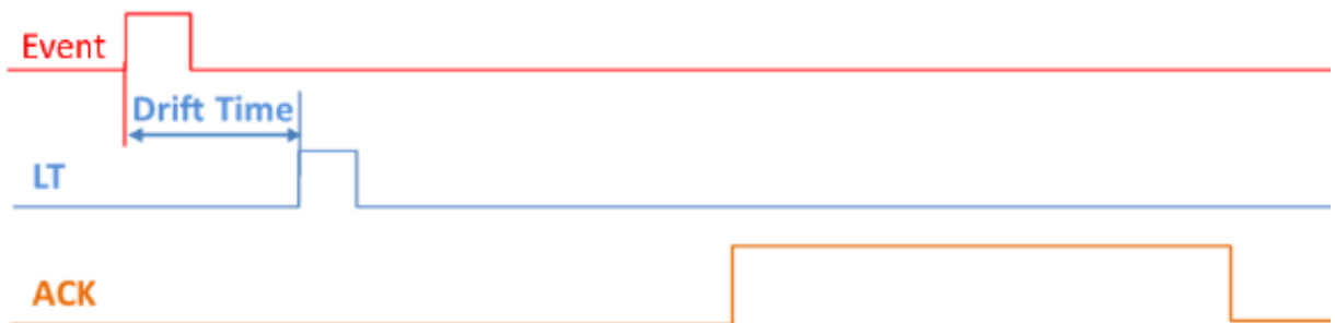
Figure 4.12 DAQ timing sequence for a single event
