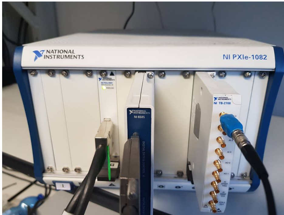
Figure 3.12 National Instrument PXIe-1082. This box is equipped with an FPGA (middle connector) and an ADC (rightmost connector) module. The left connector is the link with the PC.
