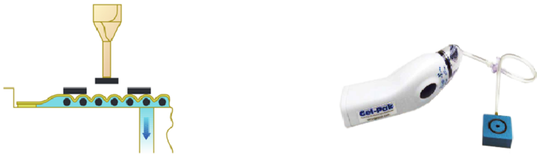
Figure 3.3 Cross-Sectional view illustrating vacuum release technology (left), vacuum pump (right)
