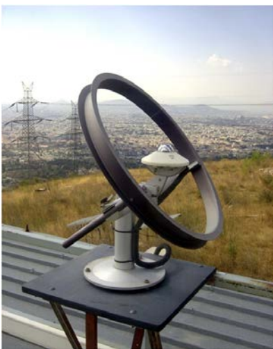
Figure 4.4 - Photo of a pyranometer
