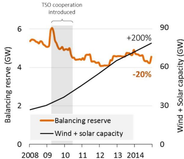
Figure 3-10 The German "paradox": Secondary + Tertiary Reserves with respect to Wind + Solar capacity [90]
