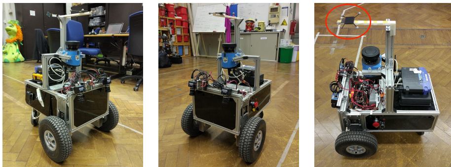
Figure 7.18: The Robocom robotic platform. The OptiTrack marker is highlighted in red in the rightmost image.
