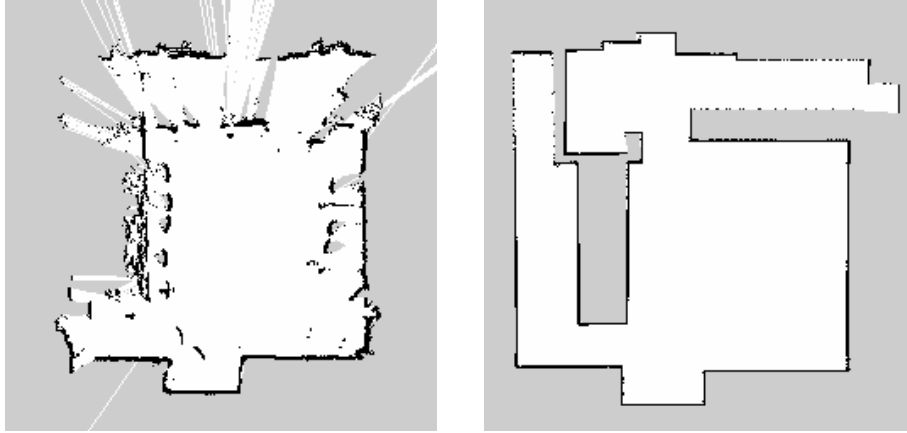
Figure 7.19: On the left, the map produced by GMapping on an autonomous exploration of the AIRLab laboratory. On the right, the map produced by GMapping on a simulation performed with the realistic simulation setting on the laboratory floor plan.
