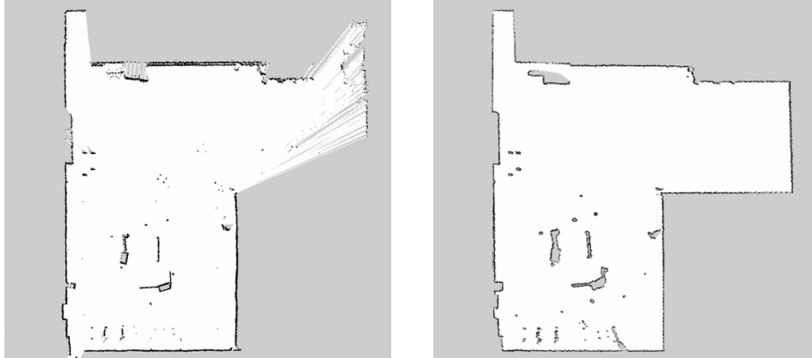
Figure 7.16: On the left, the map produced by GMapping using the recorded sensory information of the dataset. On the right, the map produced by GMapping on a simulation performed with the same robot setting used to gather the original dataset.
