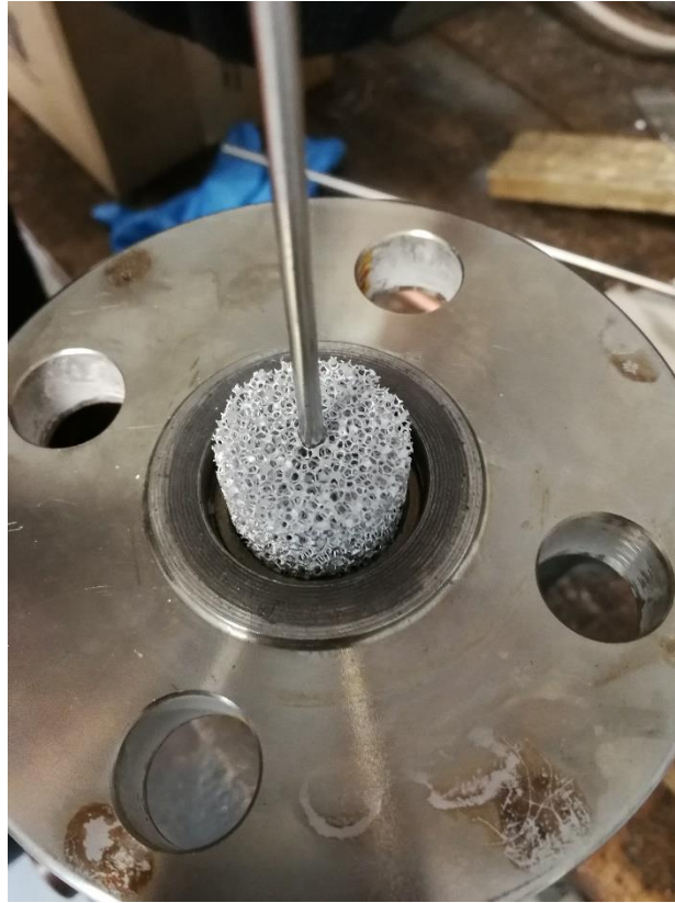
Fig. 4.9: Foam loading into the reactor.
