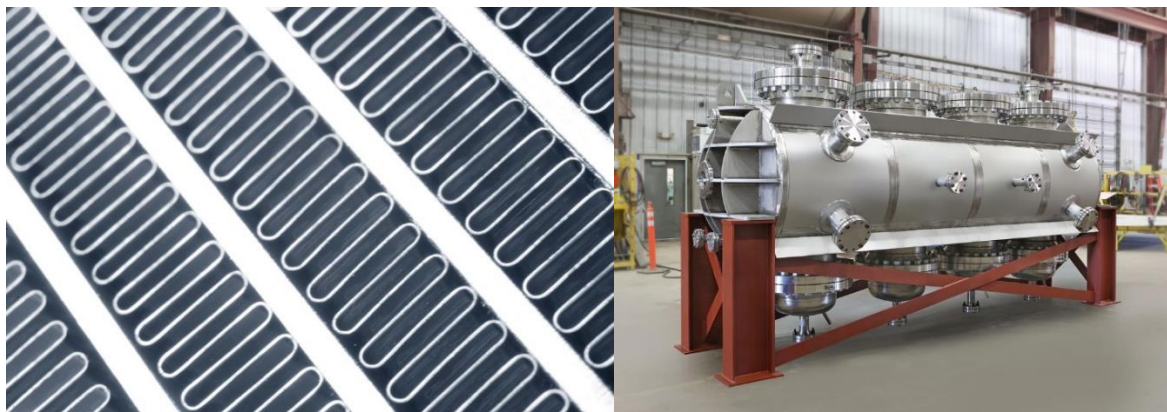
Fig. 4.2: Segment of a microchannel (left) and a three microchannels FT reactor within a pressure vessel (right) with Velocys approach. [27]
