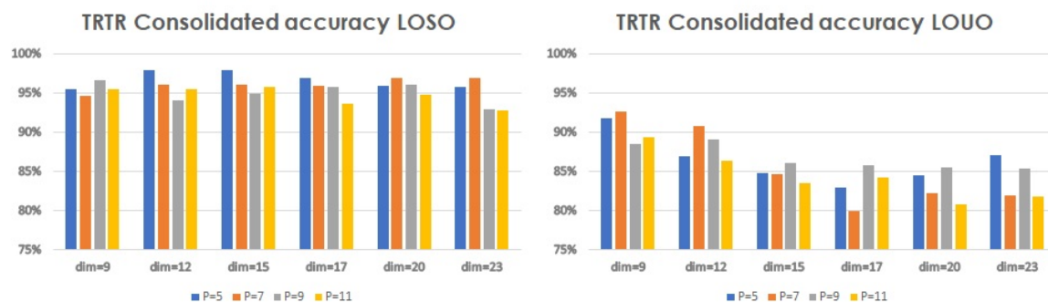
Figure 4.5: Performances of the TRTR are studied in terms of overall consolidated accuracy. This metrics computed through Equation (3.33) is studied for every combination of concatenation length ( P ) and number of features ( dim ) on the LOSO and LOUO validation schema.
