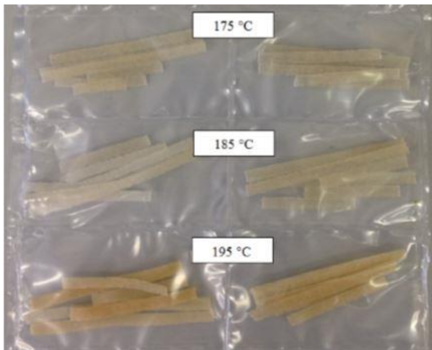
Figure 6.1: Extruded ribbons for temperatures ranging from 175 to 195°C and for rotation speeds of 30 (on the left) and 100 rpm (on the right)
