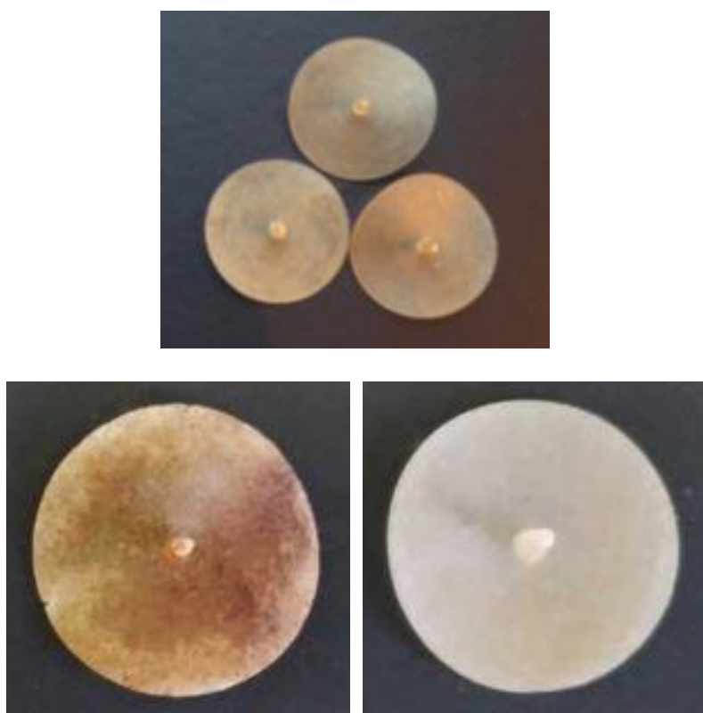
Figure 6.6: Micro injection moulded disks of KIR (on the top), Pullulan (on the left) and dried and co-milled Pullulan (on the right)
