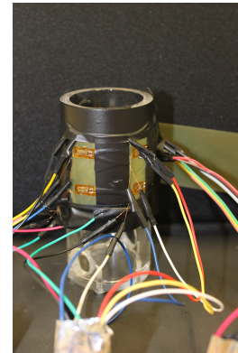
(b) Probe with D = 50 mm in test configuration
