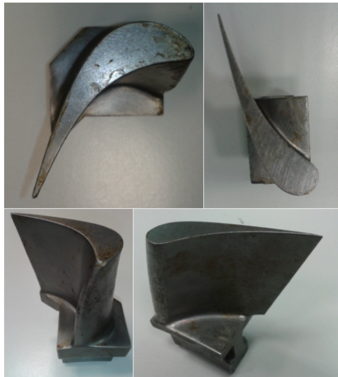
Figure 4.12: Prototypes of the rotor blades on the left, and stator blades on the right.
