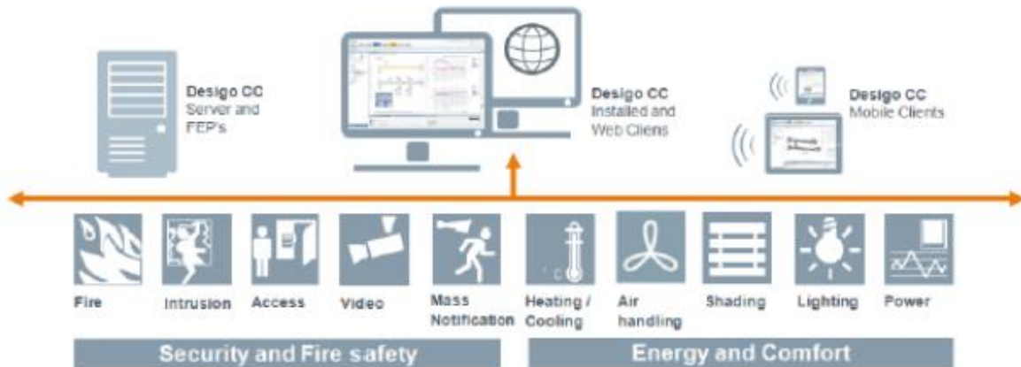
Figure 32 - BMS schematic Centralized – Source: Artelia
