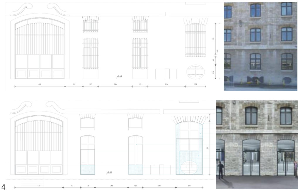
Figure 2.30 Openings enlarged to become shop windows on the street - Source: Constructa Urban Systems, 2013, Les Docks Roadbook Version 2.0
