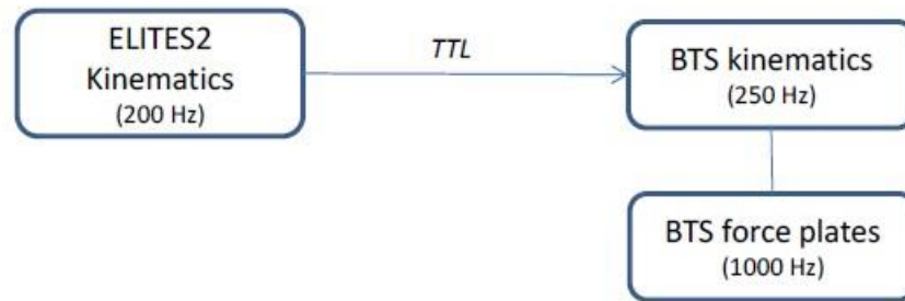
Figure 2. 4 Sync TTL signal generated by ELITES2 and read out by the BTS system to correlate GRF data
