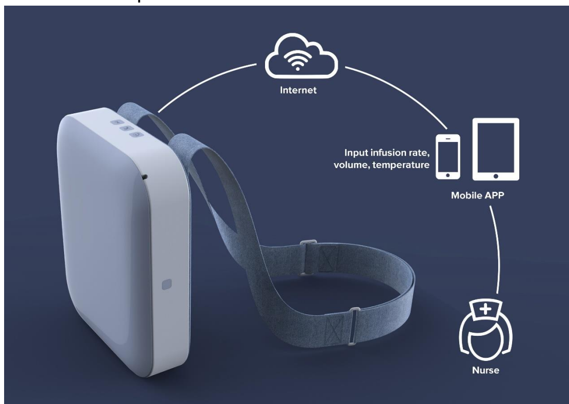
-Fig.87 Wifi Control Principle made by author
