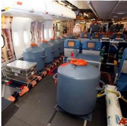
Figure 9. Ballast barrels in Airbus A380 at Paris Air Show [10]
