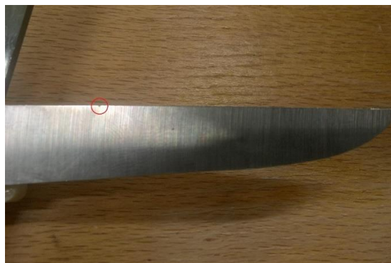
Figure 3.17 Nick on the blade
