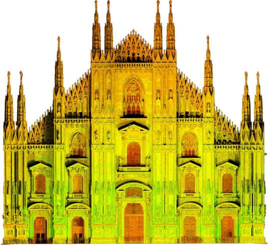
2.62 Point cloud of the façade scanned by 3DSG
