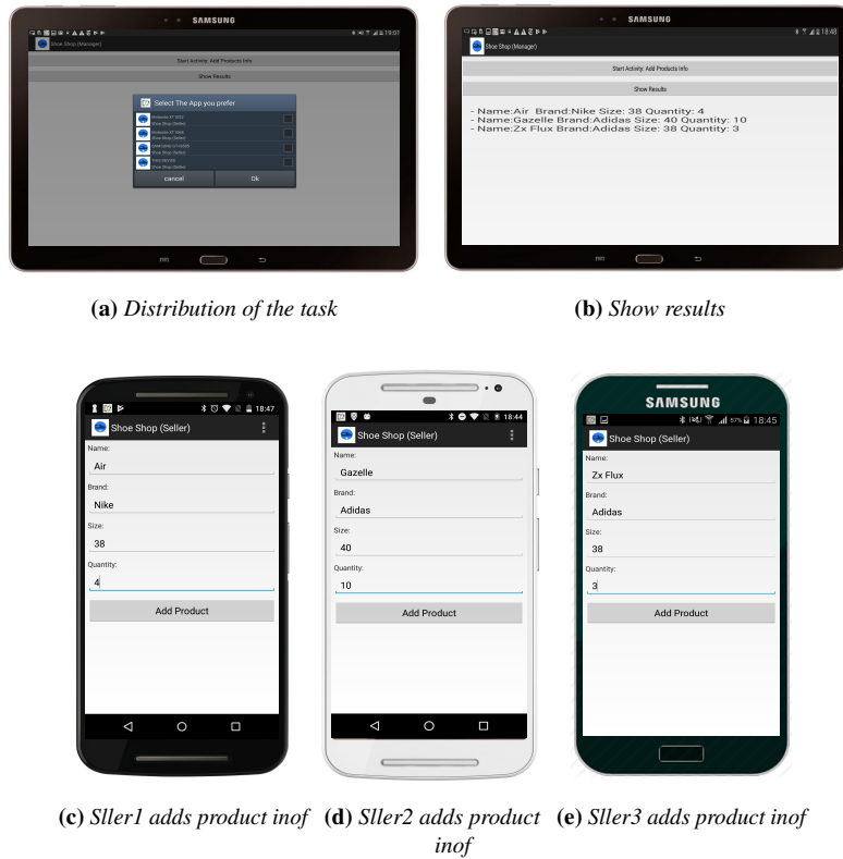
Figure 6.8: (a) The user selects to launch the activity to add products on the Sellers’ devices. (c)(d)(e) The selected sellers will add the product info in the launched activity through their devices. (b) The manager later is able to apply query and view all the inserted results through LIQDROID in the database on his device.
