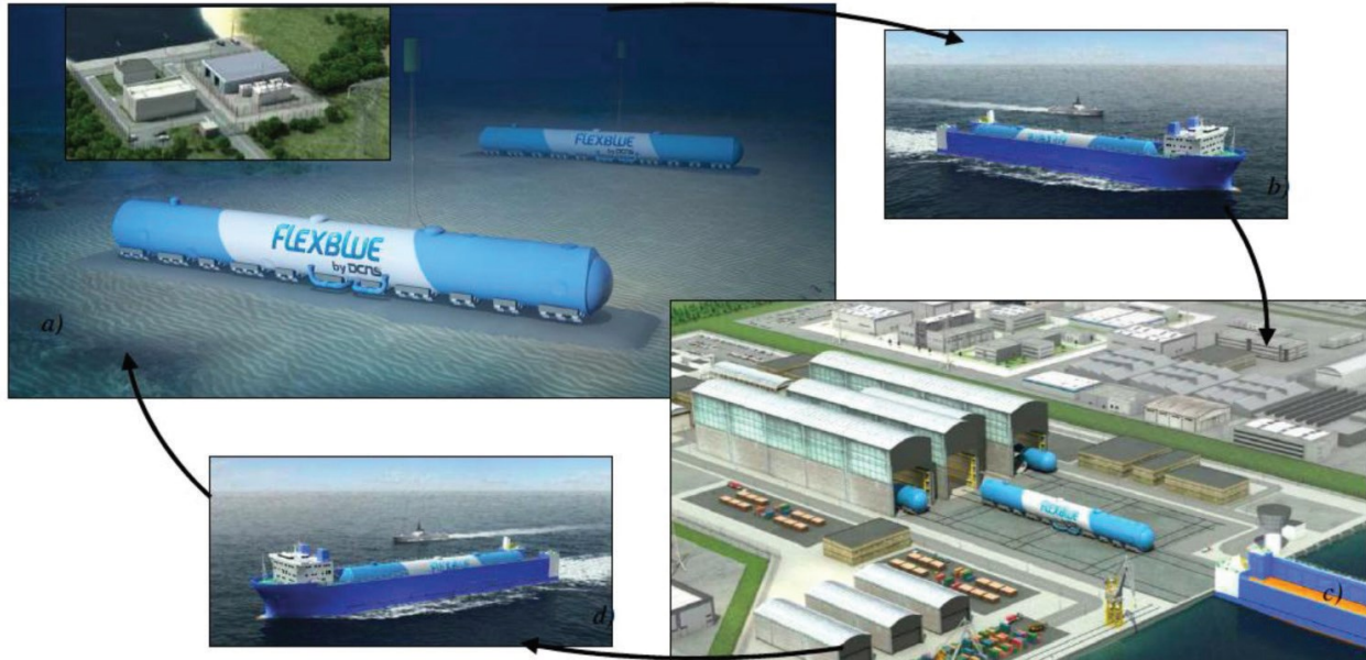
Figure 104 Artist views of a Flexblue module lifecycle: a) the subsea production site and the onshore control center; b) the ship transport; c) the support facility for refueling and maintenance; d) the transport back to the production site. (Gourmel, et al., 2016)
