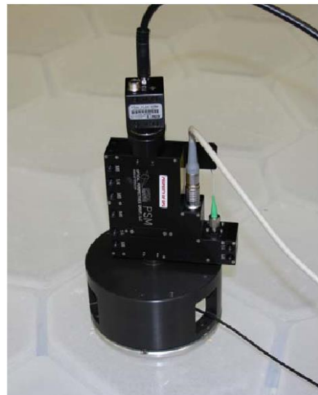
Figure 5.16 Left: optical scheme of the PSM. Image from [5.28] Right: MFT measuring the primary mirror of the Giant Magellan Telescope. Image from [5.29]
