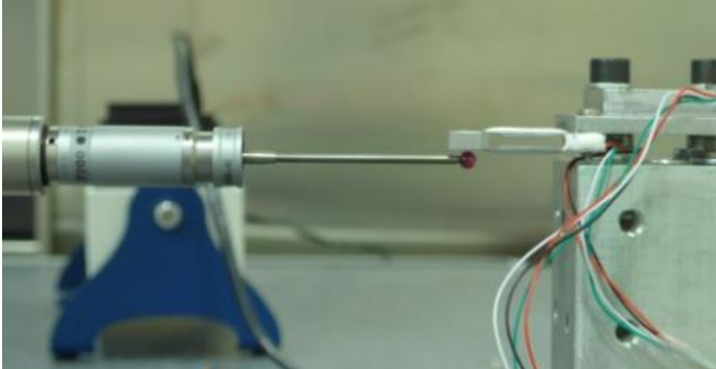
Figure 4.26. Example of force acquisition in radial direction. In this case the probe is composed by an L50D4 stylus (Renishaw code A-5003-0045) and a Standard Force module and both the altitude and clock axis at 90°. The acquisition is performed in the +Z direction meaning that the ram is moving against the gravity.
