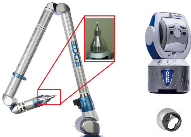
Figure 4.40. Manually operated measuring machines. Left: AACMM and a detail of the probe. Right: Laser tracker vantage and an SMR.
