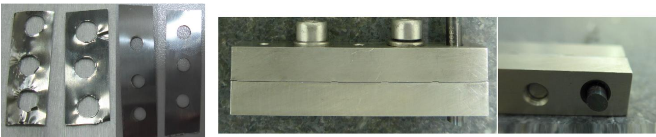
Figure 2.20 Left: Holed shims obtained by punching: from left to right 0.02, 0.05, 0.1 and 0.2 mm. Right: one of the puncher used.
