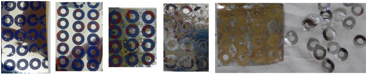
Figure 2.22 Different phases of the shim production with etching. Left to right: print with press and peel paper, correction of the print with a permanent marker, foil after the etching process, removal of the print, final shims after 30 minutes of acetone bath.
