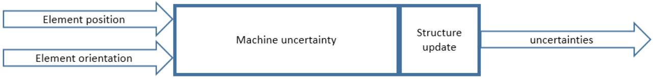
Figure 3.58 General view of the machine uncertainty module. The machine uncertainty' calculates the uncertainty based on the location and the orientation of the element while the 'structure update' takes the results and organize them in the uncertainties structure.
