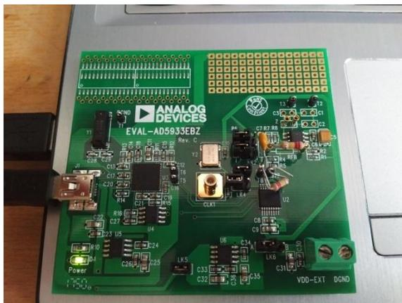
Figure 38: Calibration setup of the EvalAD5933EBZ board
