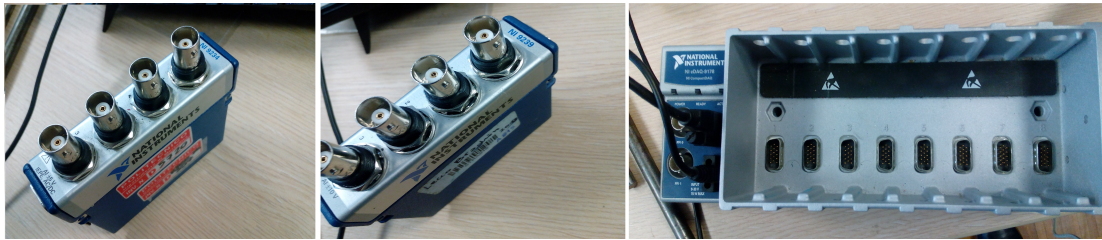
Figure 3.24: Sensors modules and data Acquisition chassis left: laser transducers module middle: accelerometer module right: modules rack.
