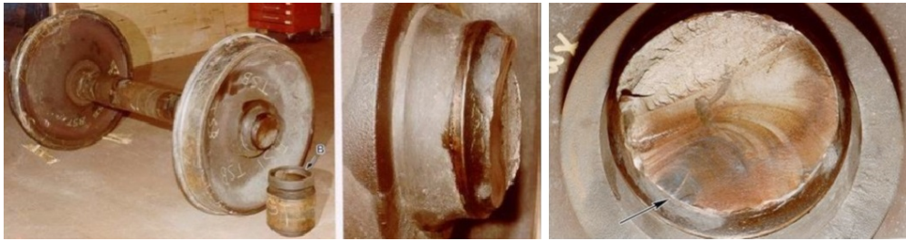
Figure 2.3: Broken axle of the Canadian accident, 2001, and zoom in the fatigue failure surface.
