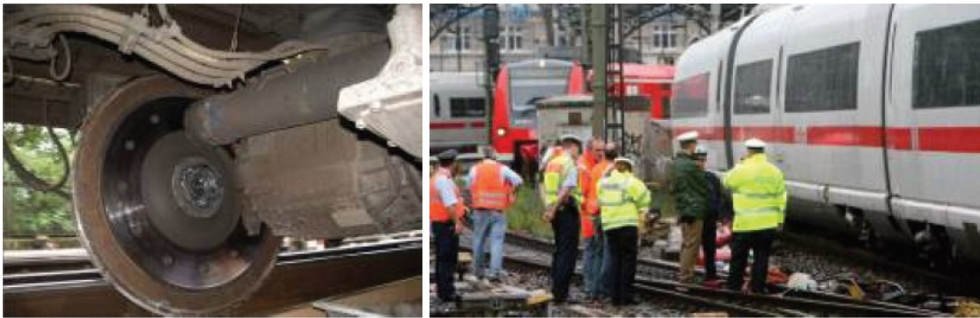
Figure 2.4: Broken axle of the IC518 ICE3 train in the Koln main station, 9.7.2008. (left: the broken driving axle seen from the internal side, right: investigators looking at the derailed train [22]).
