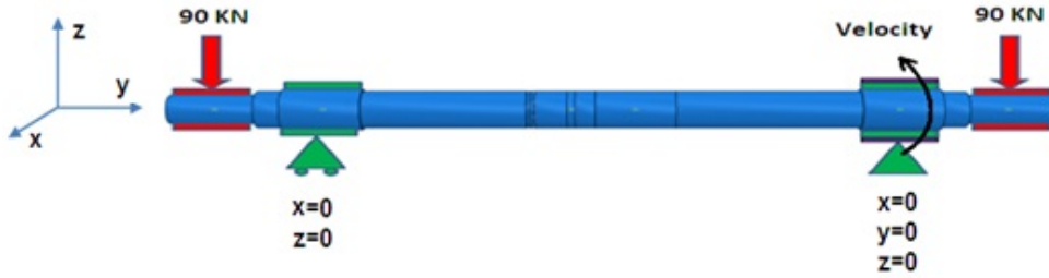
Figure 3.5: "Second case" model with simple support BCs and loads applied at the axle ends.
