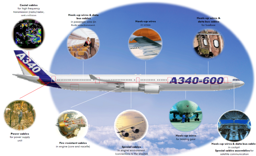
Figure 1-4. A map showing different cable types with their function in an Airbus A340 aircraft [3]
