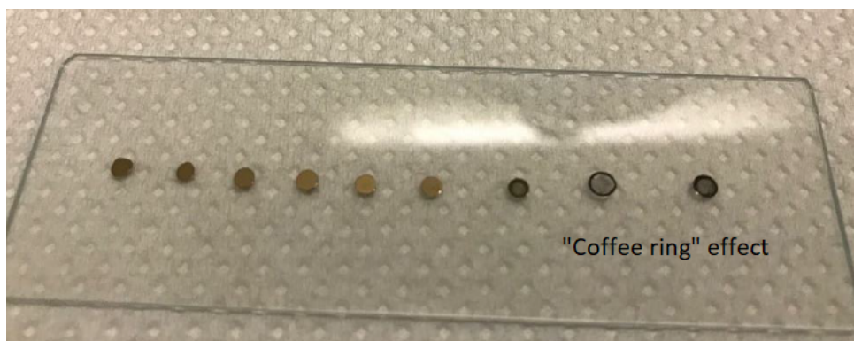
Figure 3.6: Chemically produced Au nanoparticles deposited on a glass support. The coffee ring effect is shown on the substrates on the right.
