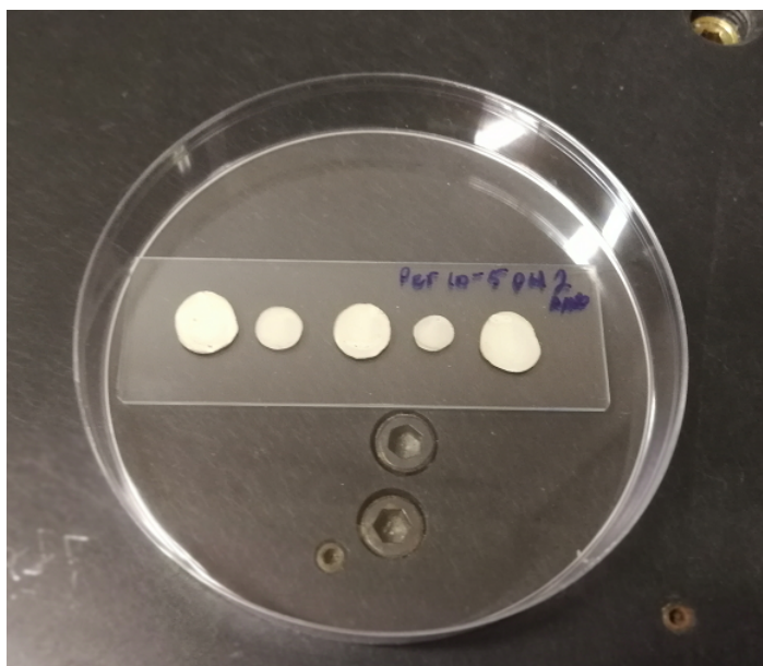
Figure 3.5: Chemically produced Ag nanoparticles deposited on a glass support.
