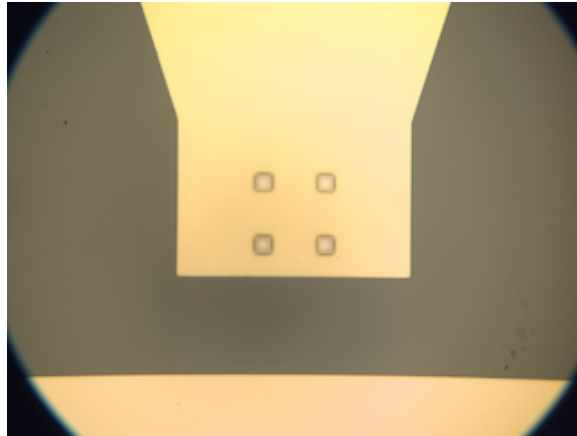
Fig. 2.6: Picture of a lithographically defined via.
