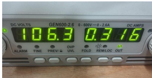
Figure 5- 7: Voltage and Current of IM running in open loop with 50 Hz of rotating field frequency
