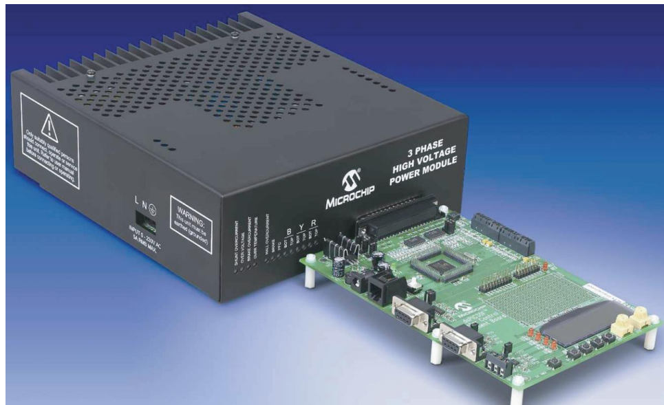
Figure 4- 5 : MC1H 3-Phase inverter connected to a microcontroller-based Platform
