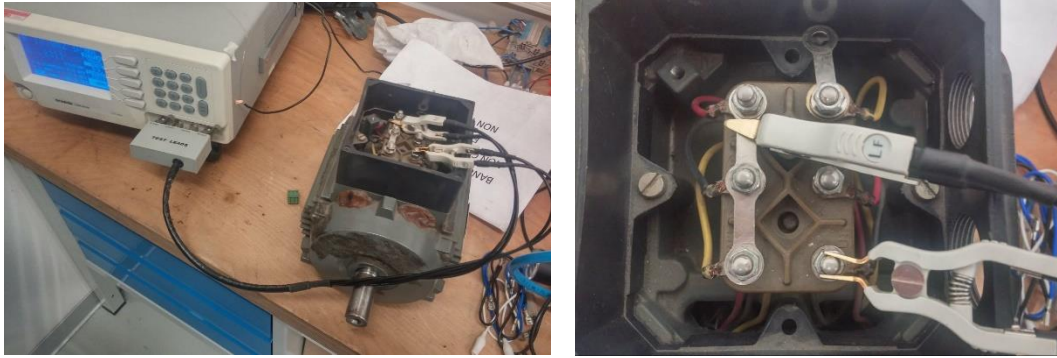
Figure 5- 5: measuring the stator resistance of Induction Motor under tests
