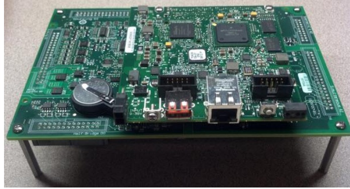
Figure 4- 4: Stacked sbRIO 9606 on GPIC 9683 mezzanine card
