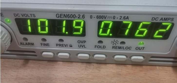
Figure 5- 10: The Voltage and Current drained from DC power supply during rotor blocking test
