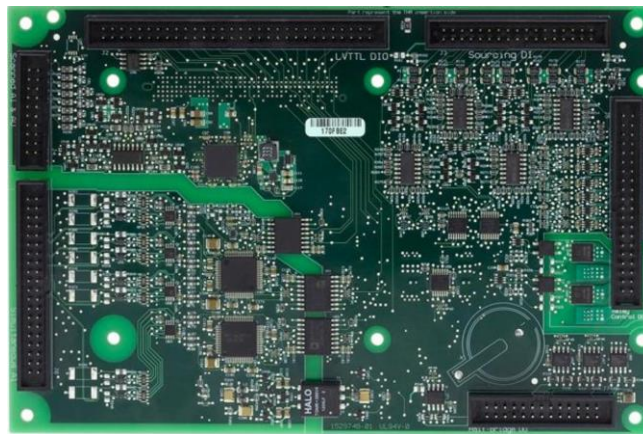
Figure 4- 3: Top view of GPIC 9683 mezzanine board
