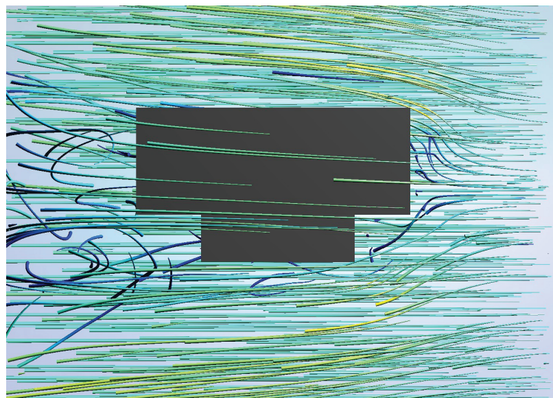
1. CFD modelling used to predict air flow pattern around Torre GALFA
