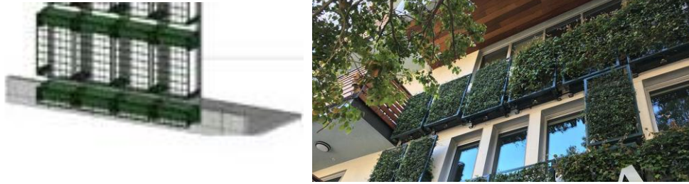
Fig. 5.6.9. Example Green Wall System
