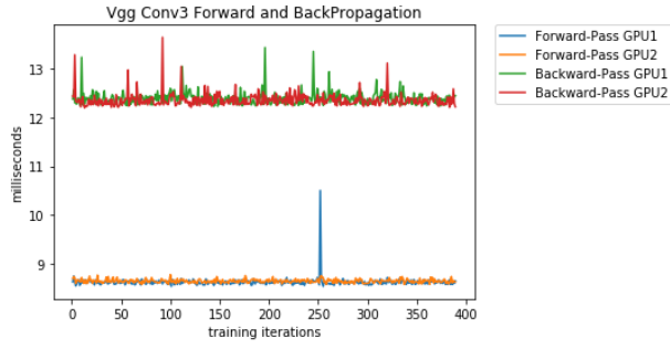
Figure 4-33 VGG Conv3 Layer-Time vs number iteration
