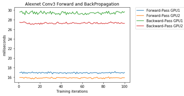
Figure 4-20 Alexnet-128 Conv3 Layer-Time vs number iteration
