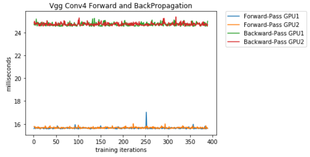
Figure 4-32 VGG Conv4 Layer-Time vs number iteration
