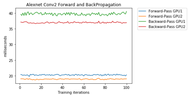
Figure 4-15 Alexnet-128 Conv2 Layer-Time vs number iteration
