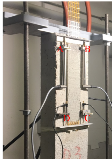
Figure 17 positioning of the LVDTs
